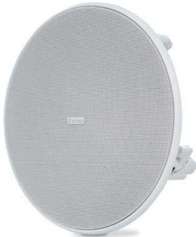
The Extron CS 3T is a full-range ceiling speaker featuring an open back design with a transformer for use in non-plenum airspace environments. It features a 3" (7.6 cm) full-range driver and can be used in 70/100 volt or 8 ohm operation. The CS 3T provides an extremely wide 165° conical dispersion for flexibility in speaker spacing. It is designed for applications where high intelligibility and maximum coverage is desired in voice reinforcement applications and low ceiling installations.
