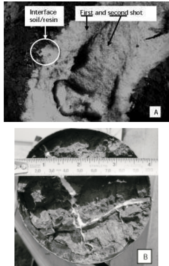
FIGURE 1: VIEW OF SOIL/RESIN COMPOSITE MATERIAL. (A) RESIN INJECTION IN SILTY CLAY. WIDTH OF THE RESIN LAYER ABOUT 20 mm. (B) RESIN INJECTION IN RESIDUAL CLAY.
