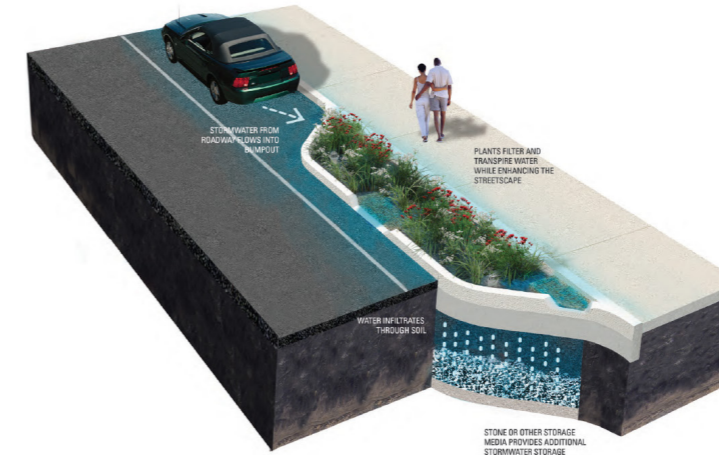
Mid-block Stormwater Bump-out
